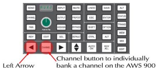
Figure 18 - Channel banking in the Master Control Panel of the AWS 900 console.
