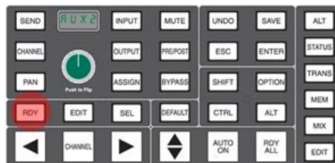
Figure 13 - RDY - Record Ready button on the Master Control Panel of the AWS 900
