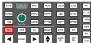
Figure 10 - RDY - Record Ready button on the Master Control Panel of the AWS 900
