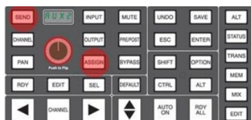
Figure 19 - Assign and Send controls, and Push to Flip button on the Master Control Panel of the AWS 900 console
