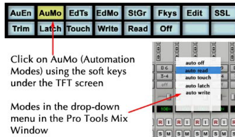
Figure 23 - Automation Mode controls on the TFT screen of the AWS 900, and corresponding drop-down menu in Pro Tools
