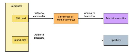
The video conforms to DV format and feeds through the 1394 card to the DV device (camcorder or DV-to-analog media converter). The DV device sends analog output to the television monitor.
