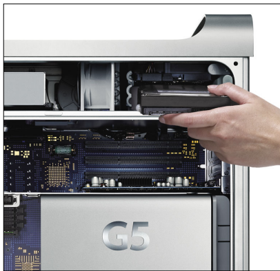
To install a new hard drive, just attach the drive guides and slide the drive onto the tracks until it clicks into place.
