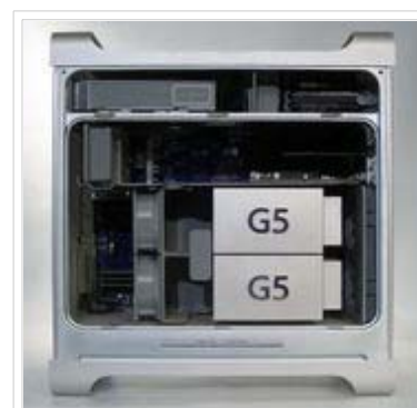
The inside of a Power Mac G5 Dual 1.8 GHz
