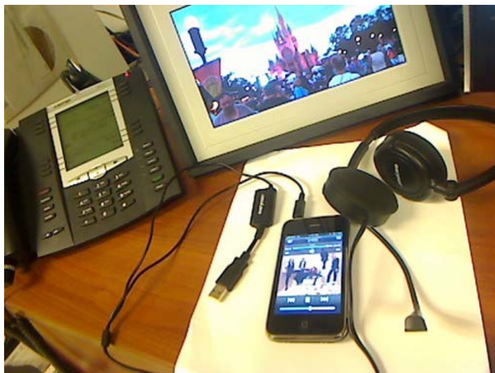
Notice the Y-cable (USB + 3.5mm jack) with the 3.5mm jack connected to iPhone
